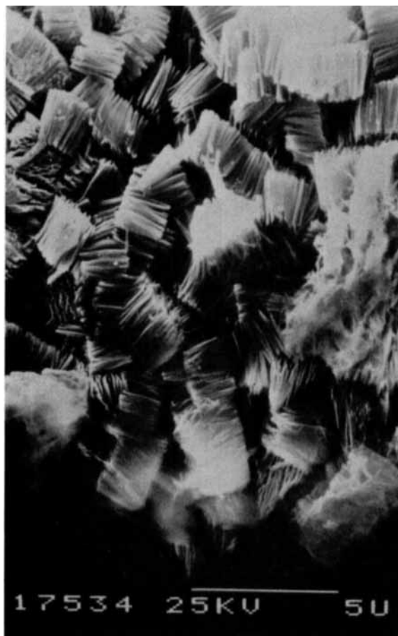
FIG. 3. PHBA accordionlike superstructure.
